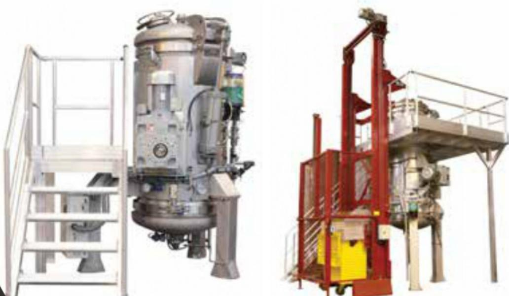
The T1000 device is distinguished by its ability to process various types of medical waste, including sharp materials such as needles, surgical gowns, and disposable medical tools. These devices are designed to provide maximum safety in the disposal of medical waste in accordance with environmental and health standards.
